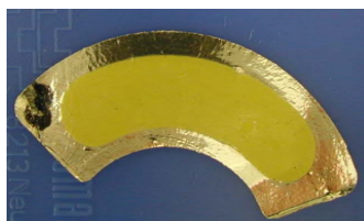
Figure 1: ^{238}\text{U} -target ( 265 \mu\text{g}/\text{cm}^2 ) produced by molecular plating of uranyl- nitrate from isobutanolic solution.
