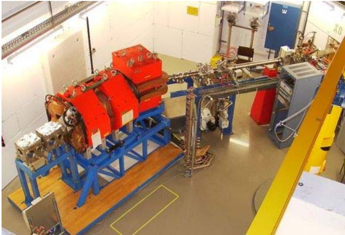
Fig. 1: View (from right to left, beam direction) of the end of the X8 beam line, the dipole the two quadrupole magnets (red), and the two detector chambers.
