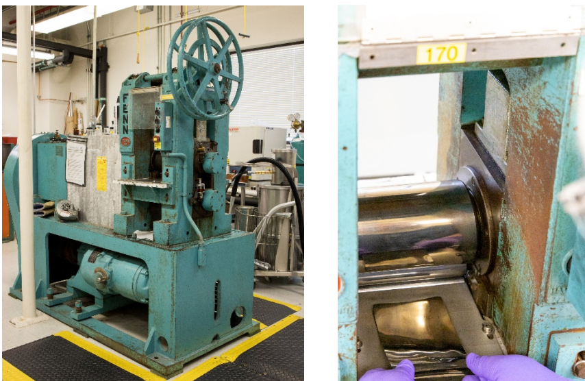
Figure 3: Left: the Fenn rolling mill. Right: rolling a foil in a stainless steel pack.
