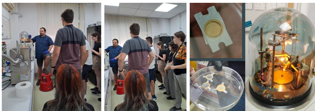
The Al foils prepared by participants were covered with a thin gold layer by PVD via resistive heating.
