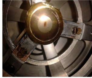
^{40}\text{Ca} (0.5 mg/cm 2 ) sandwiched between Au reduction & PVD
