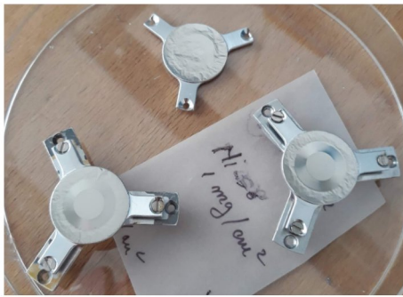
^{58}\text{Ni} (1 mg/cm 2 ) cold rolling
