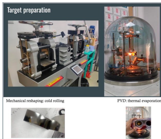
Target preparation, featuring hands-on experience with cold-rolling and PVD techniques (images from the participants' final reports).
