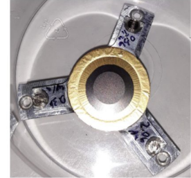
^{46}\text{Ti} (0.36 mg/cm 2 ) / Au reduction & PVD
