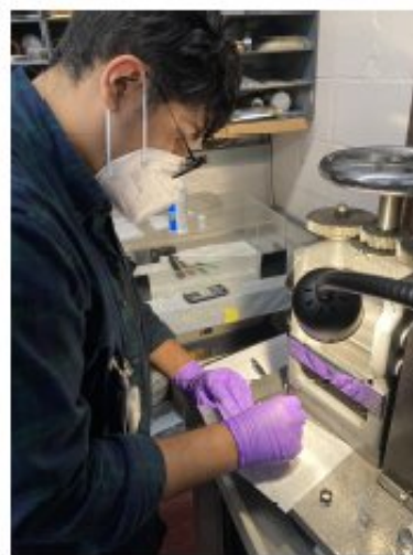
Figure 1: Photo of J. Diaz rolling the ^{54}\text{Ti} target using the CATS rolling mill.
