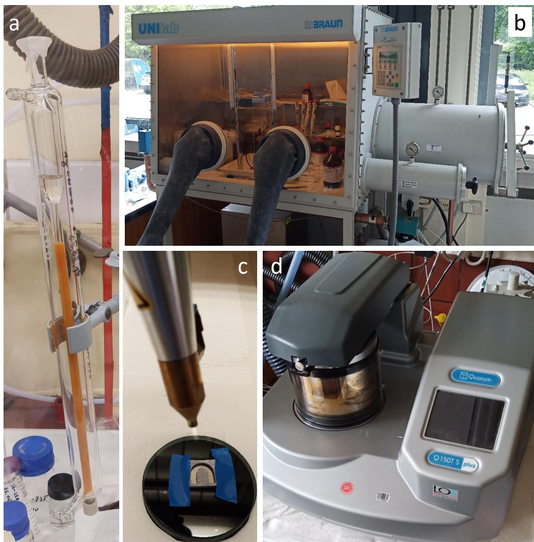
Figure 3: (a) Picture of a typical column used for chemical separation of unwanted contaminants or to separate daughter nuclides from the desired nuclide of interest. (b) An argon glove box used to store water-free solvents or to conduct experiments under controlled conditions. (c) A commercial sputter coater (Q150T from Quorum) to cover substrates or targets with thin metallic layers. (d) A commercial plasma torch (PlasmaBeam Mini from Diener Electronics), that can be used for cleaning of surfaces or to increase hydrophilicity of substrates.
