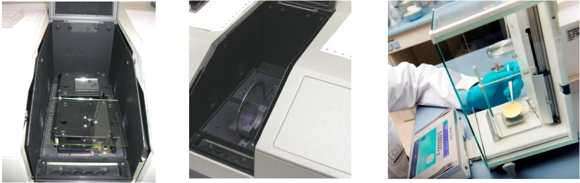
Figure 6: (Left) Measuring the areal density of the polyimide foil on the glass plate with the visible light spectrophotometer in the light reflection mode and (Middle) of the foil transferred on the frame in the light transmission mode; Accurate weighing of a deposited layer by weighing.
