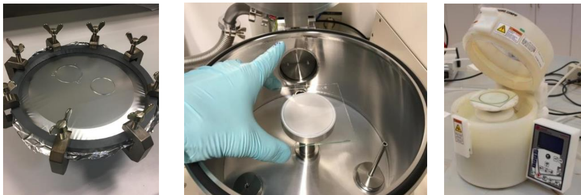
Figure 3: (Left) Stretching of an aluminium foil with a thickness of 10\ \mu\text{m} and mounting on the aluminium rings by gluing; (Middle) Pre-treating a glass plate in a low-pressure plasma cleaner to increase the hydrophilicity; (Right) Spin coater to cover the glass plate with the polycondensate solution.
