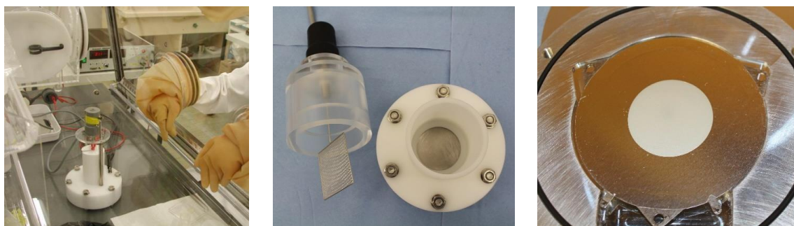
Figure 2: (Left) Molecular plating cell in a glove box; (Middle) Upper part of molecular plating cell with Pt anode and motor, and lower part in polyacetal with substrate as cathode; (Right) Layer of 99.9% ^{240}\text{Pu} with a diameter of 33 mm and a ^{240}\text{Pu} areal density of 66 \mu\text{g}\cdot\text{cm}^{-2} deposited by molecular plating. The substrate is a 0.018 mm thick aluminium foil stretched and glued on a 0.3 mm thick metal ring with inner and outer diameter of 64 mm and 74 mm respectively.
