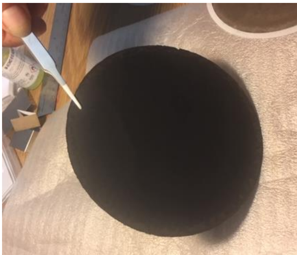
Fig. 2: 10 mg/cm 2 natural boron + 5 mg/cm 2 carbon. Disc is 12.5 cm in diameter
