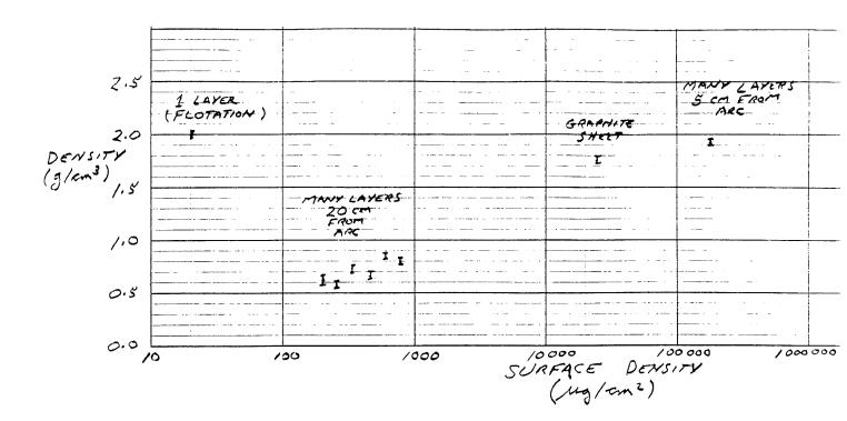
Figure 1. Densities of arc-evaporated carbon films.
