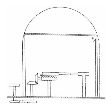
Fig. 1 Carbon-arc deposition set-up
