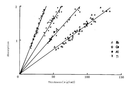
Fig. 1 Thickness calibration curves for holmium, cobalt, nickel and titanium foils as a function of their absorption of light at 680nm.
