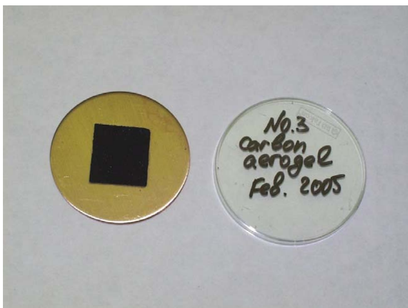
Figure 4: Carbon aerogel glued onto a copper disk.
