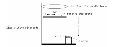
Fig.1.Schematic drawing of the rotating substrate set-up.
