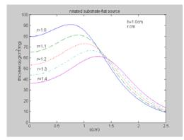
Fig.2. Theoretical film thickness distributions for a source-to-substrate distance h=1.0cm.
