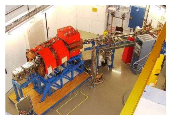
Fig. 1: View (from right to left, beam direction) of the end of the X8 beam line, the dipole the two quadrupole magnets (red), and the two detector chambers.
