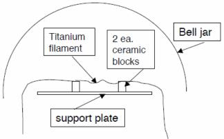
The titanium filament is type TSP-12-VA, obtained from Duniway Stockroom (<www.duniway.com>). The support plate, which prevents titanium evaporant and flakes from bombarding the apparatus below it in the bell jar, is aluminum, and the connecting leads are copper. The ceramic blocks have dimensions 19 mm x 19 mm x 25.4 mm, but ordinary porcelain standoffs used for electrical wiring would work as well.
