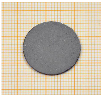
Fig. 3: Pressed tablet of enriched 62-Ni
