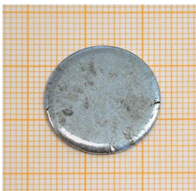
Fig. 4: Metal tablet of enriched 68-Zn
