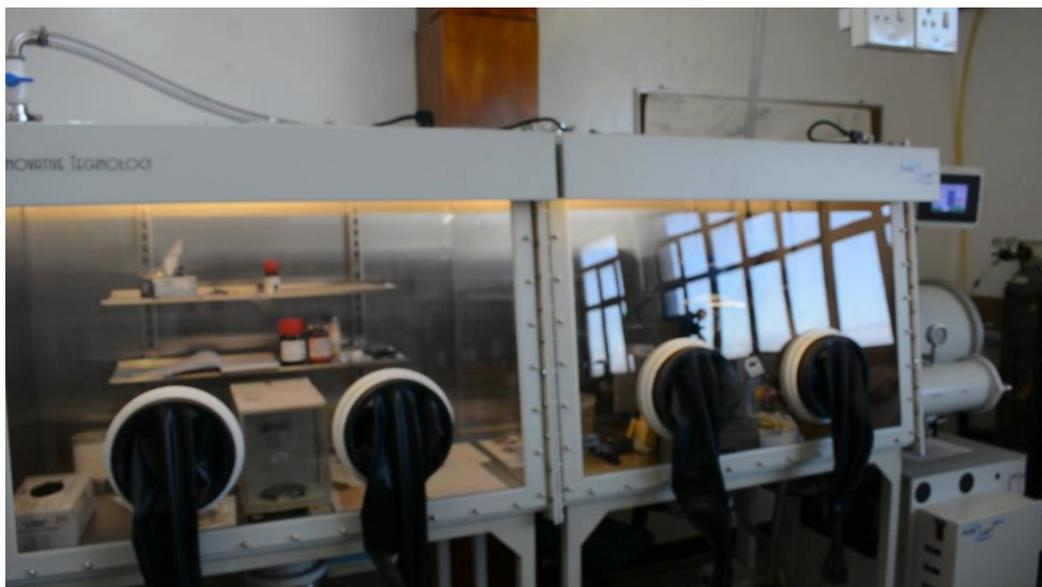
**Figure 3:** Glove box for providing inert atmosphere during manufacturing of air and moisture-sensitive targets. .
