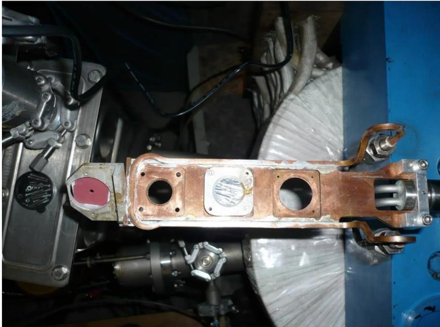
**Figure 2:** Li-target covered with Havar foil inside the experimental target chamber.
