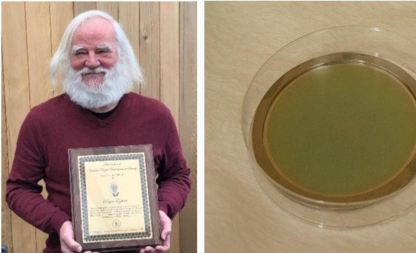
Fig 1. Left: Roger Eykens receiving the INTDS2020 Award, Right:  $^{235}\text{UF}_4$  layer with an areal density of  $67 \mu\text{gcm}^2$  prepared by physical vapour deposition on a polyimide foil with an areal density of  $27 \mu\text{gcm}^2$  coated with a  $50 \mu\text{gcm}^2$  gold layer
